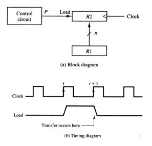
As shown in the timing diagram P is activated in the control section by the edge of a clock pulse at time t. The next positive transition of the clock at time t + 1 finds the load input active and the data inputs of R2 are then loaded into the register in parallel. P may go back to 0 at time t + 1, otherwise, the transfer will occur with every clock pulse transition while P remains active
