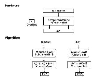
Comparing this algorithm with its signed – magnitude counterpart, we note that it is much simpler to add and subtract numbers if negative numbers are maintained in signed -2's
