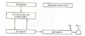
The two bits of the multiplier in  $Q_n$  and  $Q_{n+1}$  are inspected. If the two bits are equal to 10, it means that the first 1 in a string of 1's has been encountered. This requires a subtraction of the multiplicand from the partial product in AC. If the two bits are equal to 01, it means that the first 0 in a string of 0's has been encountered. this requires the addition of the multiplicand to the partial product in AC.
