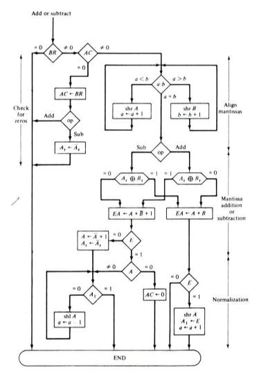
The magnitude comparator attached to exponents a and b provides three outputs that indicate their relative magnitude. If the two exponents are equal, we go to perform the arithmetic operation. If the exponents are not equal, the mantissa having the smaller exponent is shifted to the right and its exponent incremented. This process is repeated until the two exponents are equal.
