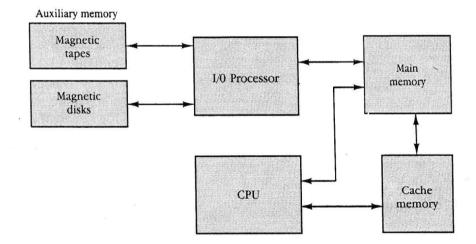
A special very-high-speed memory called a cache is sometimes used to increase the speed of processing by making current programs and data available to the CPU at a rapid rate. The cache memory is employed in computer systems to compensate for the speed differential between main memory access time and processor logic. CPU logic is usually
