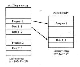
A table is then needed, as shown in Fig. 6.16, to map a virtual address of 20 bits to a physical address of 15 bits. The mapping is a dynamic operation, which means that every address is translated immediately as a word is referenced, by CPU.
