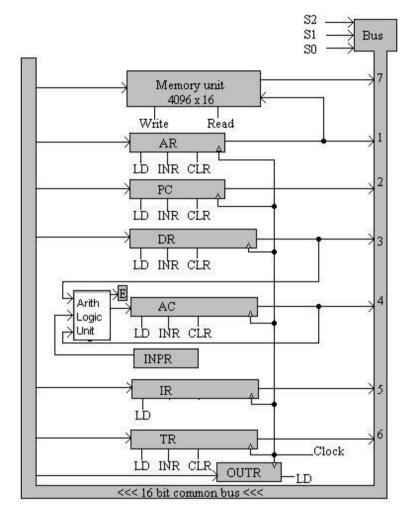
The input register INPR and the output register OUTR have 8 bits each and communicate with the eight least significant bits in the bus. INPR is connected to provide information to the bus but OUTR can only receive information from the bus. This is because INPR receives a character form and input device which is then transferred to AC. OUTR receives a character form AC and delivers it to an output device. There is on transfer from OUTR to any of the other register.
