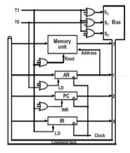
Figure 3.8 Register transfer for the fetch phase
