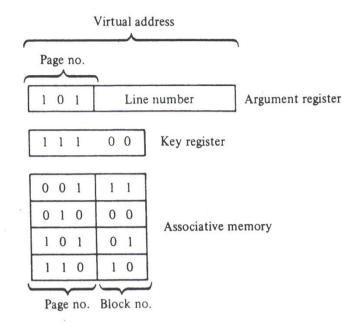
The page field in each word is compared with the page number in the virtual address. If a match occurs, the word is read from memory and its corresponding block number is extracted.
