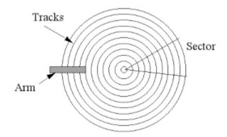
Some units use a single read/write head for each disk surface. In this type of unit, the track address bits are used by a mechanical assembly to move the head into the specified track position before reading or writing. In other disk systems, separate read/write heads are provided for each track in each surface. The address bits can then select a particular track electronically through a decoder circuit. This type of unit is more expensive and is found only in very large computer systems.
