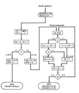
A divide – overflow condition is tested by subtracting the divisor in B from half of the bits of the dividend stored in A. If  $A \ge B$ , the divide-overflow flip-flop DVF is set and the operation is terminated prematurely. If A < B, no divide overflow occurs so the value of the dividend is restored by adding B to A.
