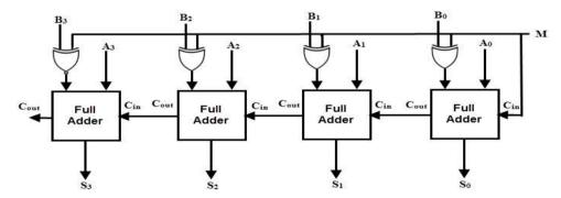
2's complement of B. for unsigned numbers, this gives A- B if A $\geq$  B or the 2' s complement of (B-A) if A< B. For signed numbers, the result is A- B provided that there is no overflow.
