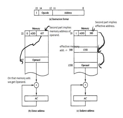
Figure 3.2 Demonstration of direct and indirect address
