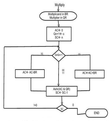
The next step is to shift right the partial product and the multiplier (including bit  $Q_{n+1}$ ). This is an arithmetic shift right (ashr) operation which shifts AC and QR to the right and leaves the sign bit in AC unchanged . The sequence counter is decremented and the computational loop is repeated n times.
