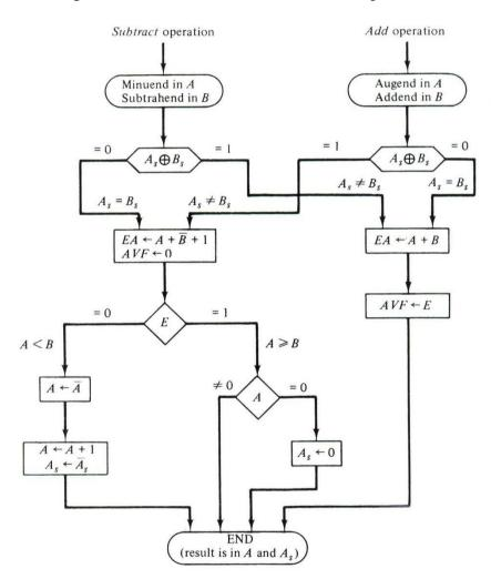
Figure 5.2 Flow chart for add and subtract operations
