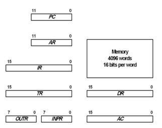
Figure 3. 3 Basic computer registers and memory
