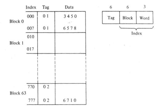
Figure 6.13 Direct mapping cache with block size of 8 words
