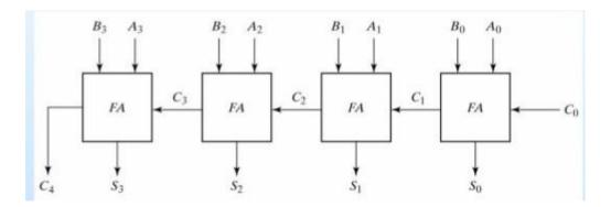
Figure 2.5 shows the interconnections of four full-adders (FA) to provide a 4-bit binary adder. The augend bits of A and the addend bits of B are designated by subscript numbers from right to left, with subscript 0 denoting the low-order bit. The carries are connected in a chain through the full-adders. The input carry to the binary adder is c0 and the output carry is C4. The S outputs of the full-adders generate the required sum bits.
