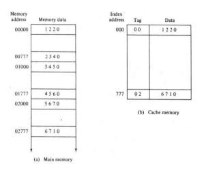
If the two tags match, there is a hit and the desired data word is in cache. If there is no match, there is a miss and the required word is read from main memory. It is then stored in the cache together with the new tag, replacing the previous value.
