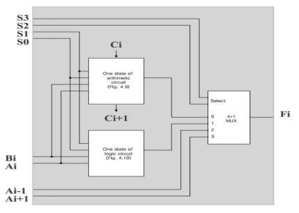
Figure 2.7 One stage of arithmetic logic shift unit
